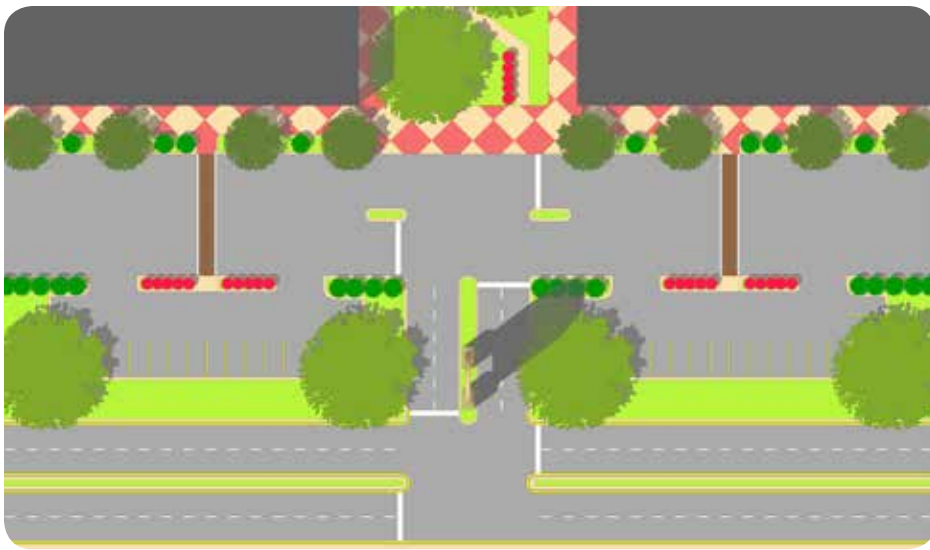
FIGURE 5.4: Diagram of shared driveways. One entrance for multiple developments encourages internal connectivity between destinations.
