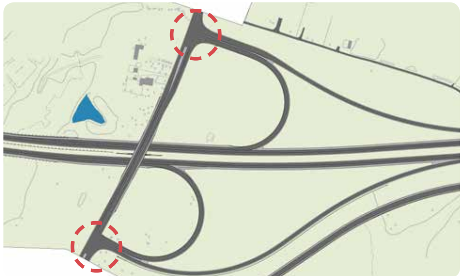
FIGURE 5.3: Location of intersections on Polkville Road that should be signalized as construction occurs on the US 74 Bypass.
