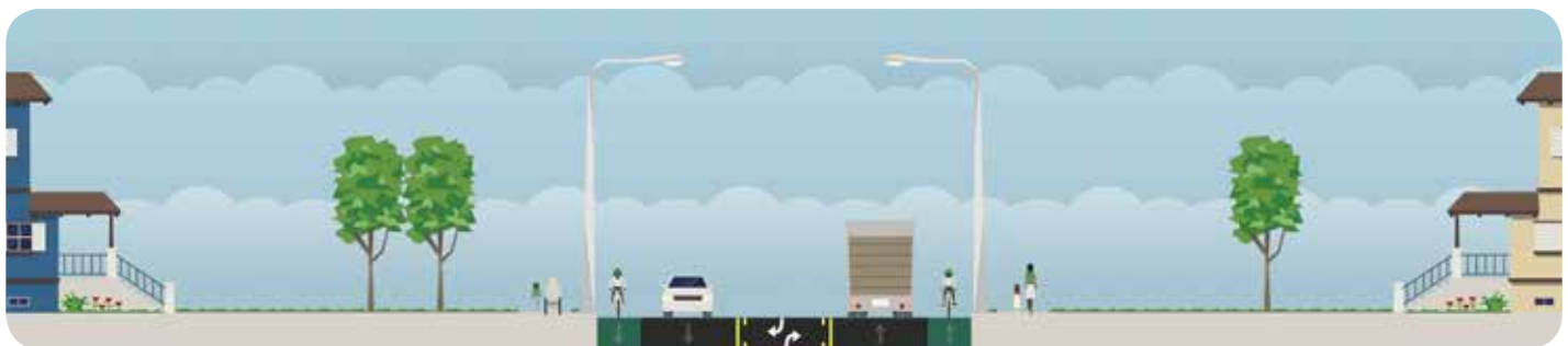
Figure 5.6: Conceptual diagram of Polkville Road as a three (3) lane road with bicycle and pedestrian amenities.
